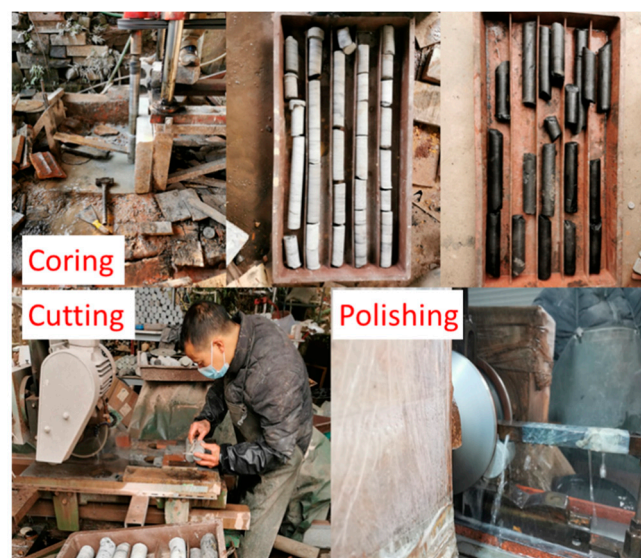
Figure 4. Processing of standard specimens.
