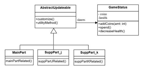
Figure 16. Class diagram of Different Parts pattern.
