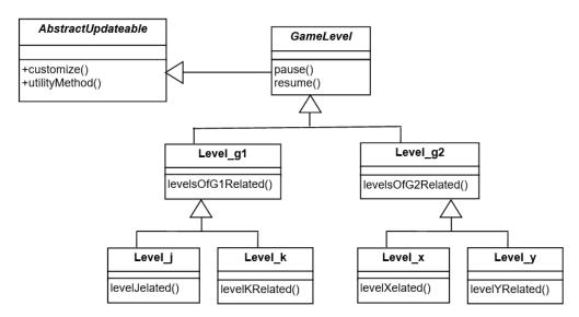
Figure 14. Second alternative approach for implementing Related Levels pattern.
