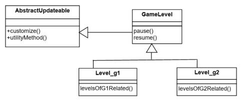
Figure 13. First alternative approach for implementing Related Levels pattern.
