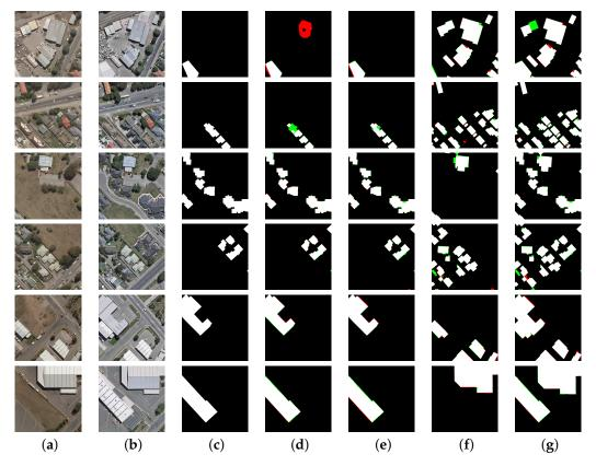
**Figure 4.** Comparative BE and CD results of two models on the WHU-CD testing set. (a)  $t_1$  image patch. (b)  $t_2$  image patch. (c) CD GT patch. (d) CD results of ChangeStar. (e) Our CD results. (f) Our BE results from  $t_1$  Image. (g) Our BE results from  $t_2$  Image. Red indicates false positives, and green indicates false negatives.
