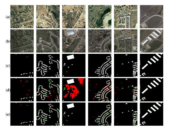
**Figure 6.** Comparative CD results on the LEVIR dataset of two models trained with the Challenge dataset. (a)  $t_1$  Image. (b)  $t_2$  Image. (c) CD GT. (d) CD results of ChangeStar. (e) Our CD results. Red indicates false positives, and green indicates false negatives.
