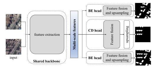
**Figure 1.** Overview of the proposed multi-task learnin (MTL) network with a shared backbone for multi-scale feature learning, two heads for building extraction, and one head for change detection.
