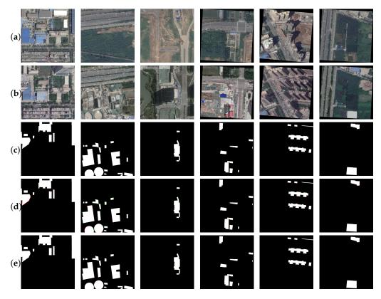
**Figure 5.** Comparative CD results of two models on the validation set of the BE and CD dataset in the Gaofen Challen (Gaofen-BECD). (a)  $t_1$  Image. (b)  $t_2$  Image. (c) CD GT. (d) CD results of ChangeStar. (e) Our CD results. Red indicates false positives, and green indicates false negatives.
