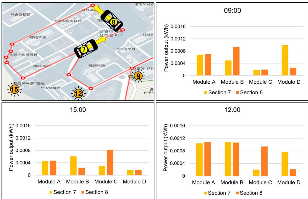
Figure 10. Comparison of PV potential by time between sections 7 and 8 in different azimuth (Korean labels in the map indicate the building name).
