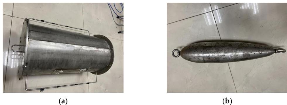
Figure 13. Experimental model: (a) cylindrical shell and (b) ballast body.
