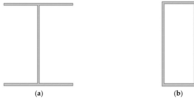
Figure 2. Section of the cross bearer of an open car frame: (a) standard structure; (b) improved structure.
