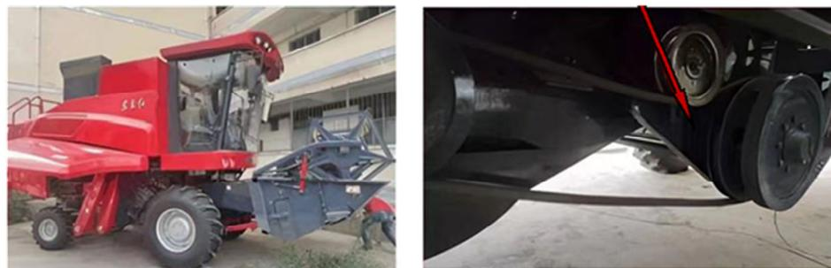
**Figure 10.** Experimental combine harvester and problem injection locations.
