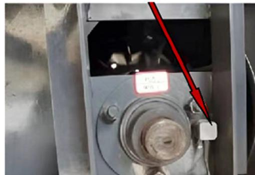
**Figure 11.** The measurement point locations of the experimental combine harvester.
