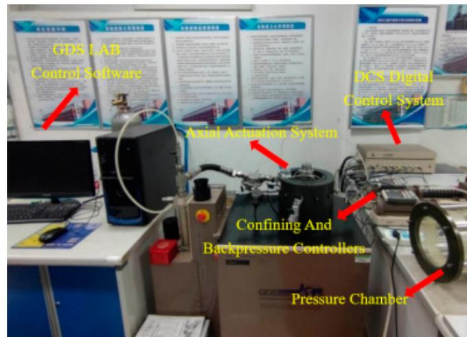
Figure 1. Dynamic triaxial testing system (DYNTTS).
