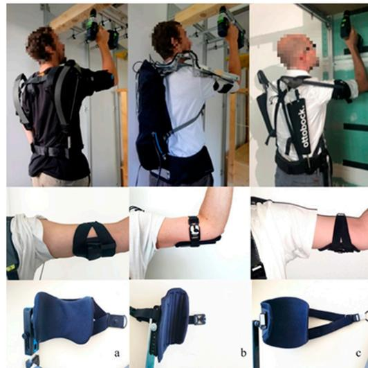
Figure 2. Exoskeletons and their pHMIs: (a) Skelex 360, (b) Lucy, and (c) Paexo Shoulder.
