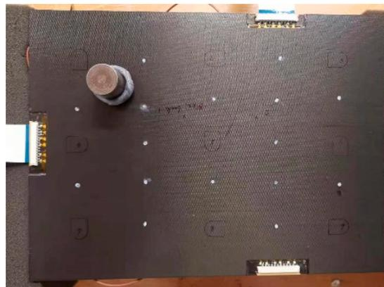
**Figure 9.** Photo of a weighted Blu Tack placed on the surface of the 2 mm thick panel.
