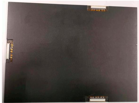
**Figure 4.** Photo of the panel with embedded PZT transducers after trimming.
