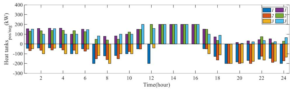
Figure 6. Positive and negative flexibility of heat tanks.
