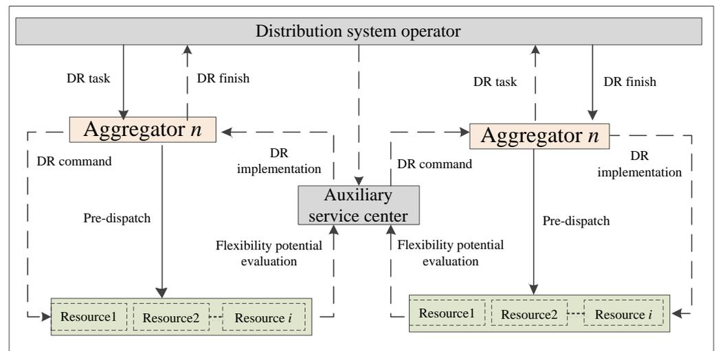
Figure 2. Functional process of the transactive DR framework.
