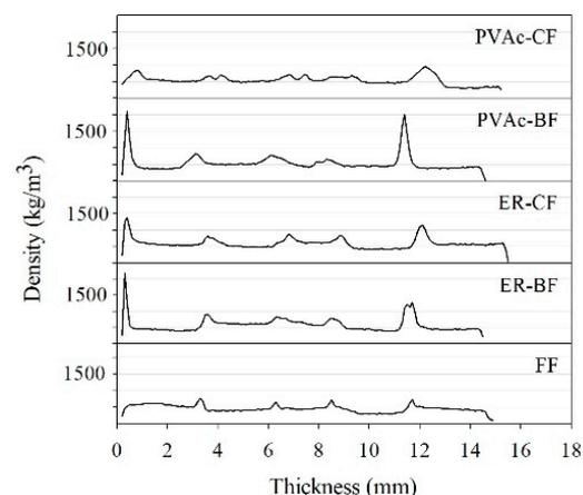
**Figure 3.** Density profile of the composite panels.
