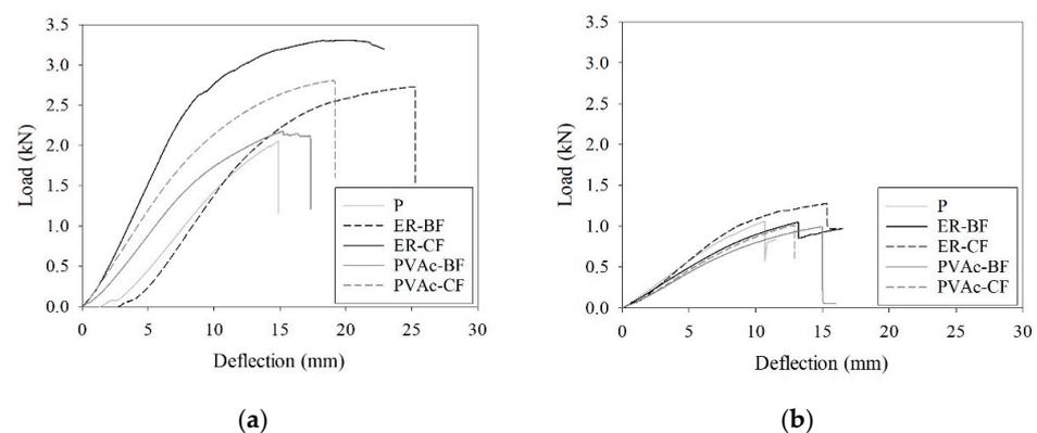
**Figure 6.** Load-deflection curves were obtained during the four-point bending test for the samples in the (a) flatwise position and in the (b) edgewise position. A characteristic curve for each sample was used as a representation of the behavior of each one.
