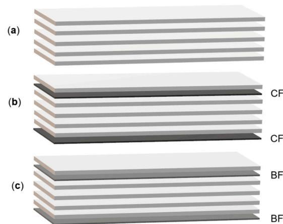
**Figure 1.** The control LVL panel, carbon fiber reinforced LVL, and basalt fiber reinforced LVL panel were configured as follows: (a) Control LVL panel; (b) LVL panel reinforced with carbon fiber; and (c) LVL panel reinforced with basalt fiber.
