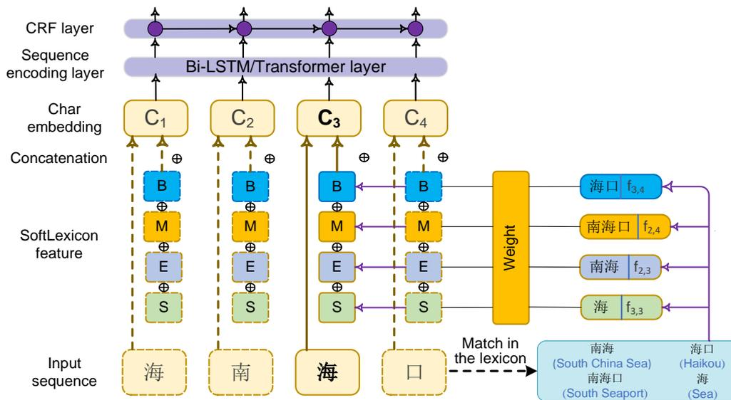
**Figure 4.** Overall architecture of the SoftLexicon model. By constructing the SoftLexicon features, the model adds the lexicon matches to the begin, middle, and end of each character, as well as single positions. Then it inputs these enhanced character embeddings into the sequence encoding layer and the conditional random field (CRF) layer to obtain the final prediction results.
