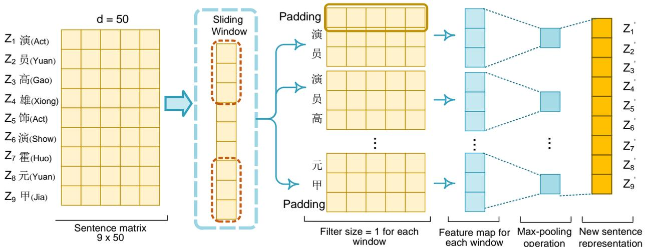
Figure 8. Short-sequence CNN with sliding window.
