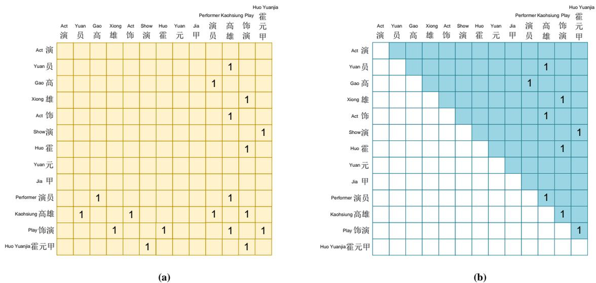
Figure 7. Optimal storage is used to hold the adjacency matrix, which depicts the connections between graph nodes: (a) original adjacency matrix and (b) optimized adjacency matrix.
