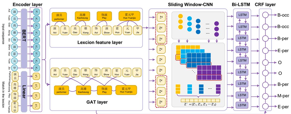
**Figure 6.** The overall proposed NER architecture. After the encoder layer, first, the sequence hidden state is obtained by short-sequence CNN combined with a Bi-LSTM structure after the fusion of the matching word information using the lexicon. Then the relationship between characters and their adjacent characters’ matching words is captured using GAT, and finally, the two outputs are summed to predict the sequence labels using a CRF layer.
