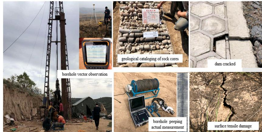
Figure 12. Field borehole observation.
