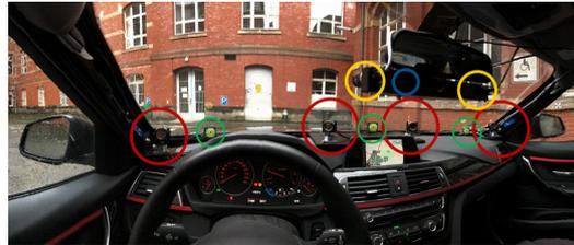
**Figure 2.** Interior of the test vehicle, with the eye tracking cameras marked by red circles, the infrared LEDs for illumination marked by green circles, the stereo camera used for part two of this series marked in yellow, and an illuminance sensor marked by the blue circle.
