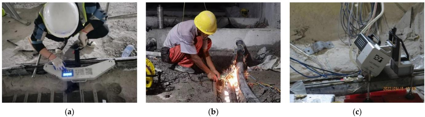
**Figure 9.** Three kinds of prestress test method: (a) transverse tension method; (b) stress release method; and (c) X-ray diffraction method.
