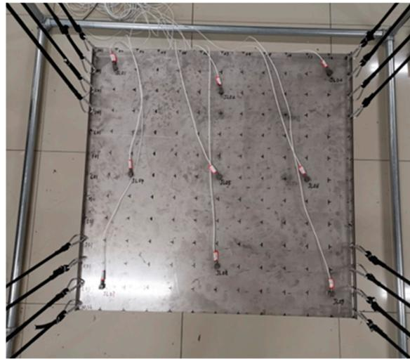
**Figure 1.** Experimental setup diagram for the suspended reinforced laminated plate structure.
