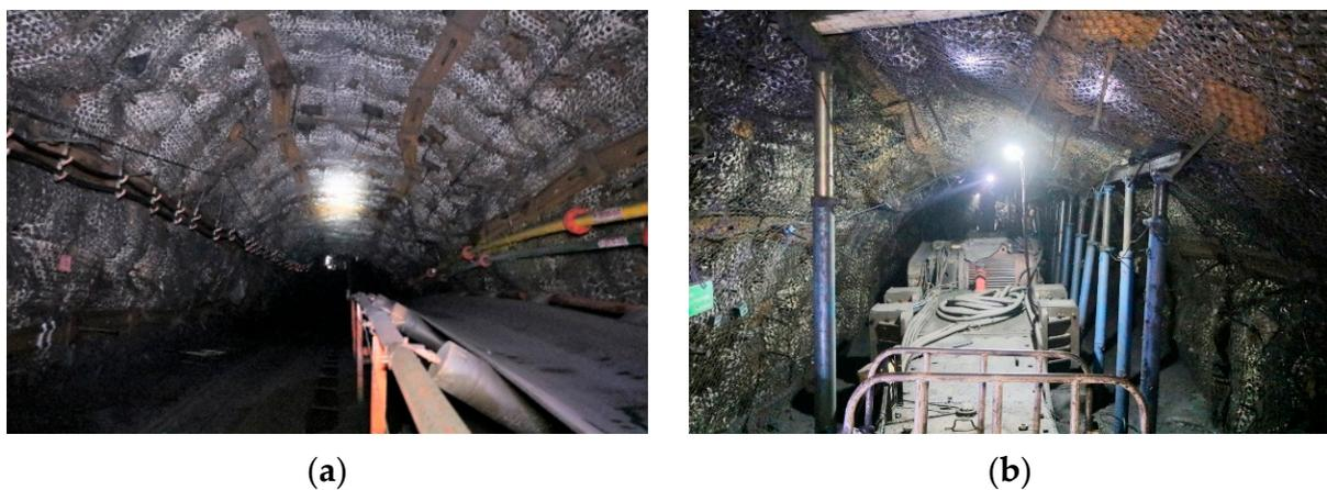
Figure 17. Roadway surrounding rock control effect: (a) During excavation; (b) During mining.
