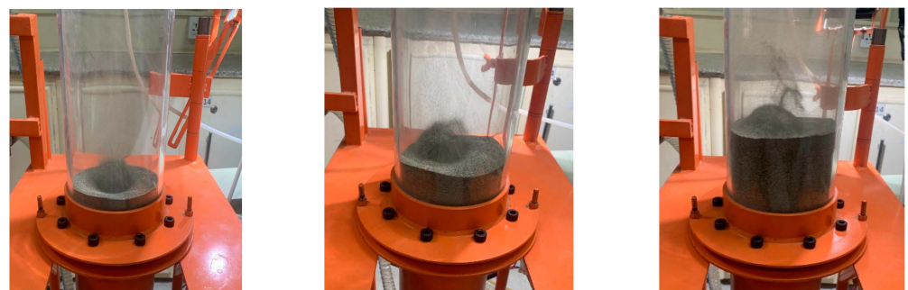
(a) Initial bed height ratio = 0.35 (b) initial bed height ratio = 0.5 (c) initial bed height ratio = 1.16
