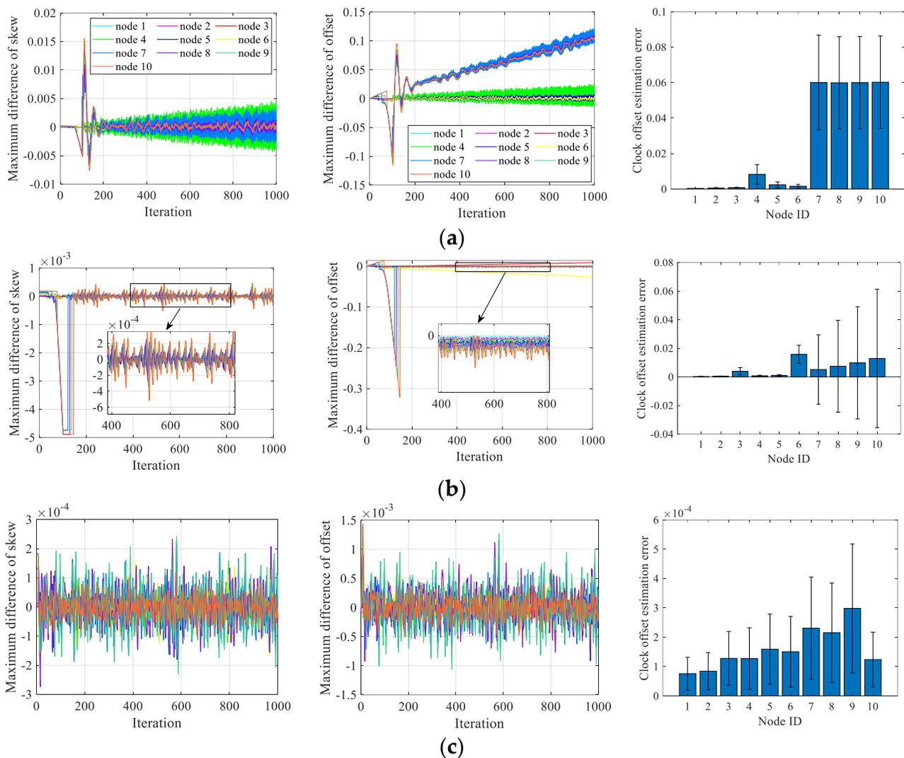
**Figure 7.** Performance of FTSP, FTSP with threshold detection, and RSTS under Sybil attacks. The representation of the lines is the same in (a–c). (a) FTSP; (b) FTSP with threshold detection; and (c) RSTS.
