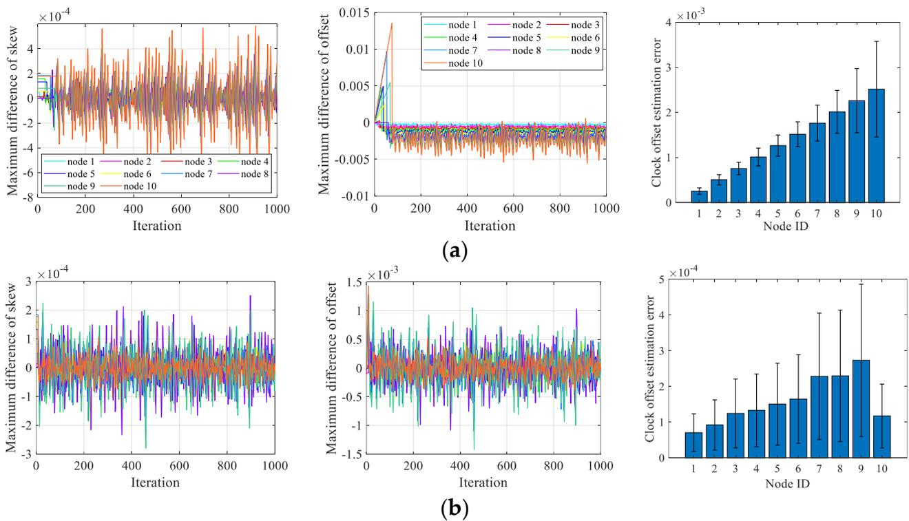
**Figure 5.** Performance of FTSP and RSTS under no attacks. The representation of the lines is the same in (a,b). (a) FTSP; (b) RSTS.
