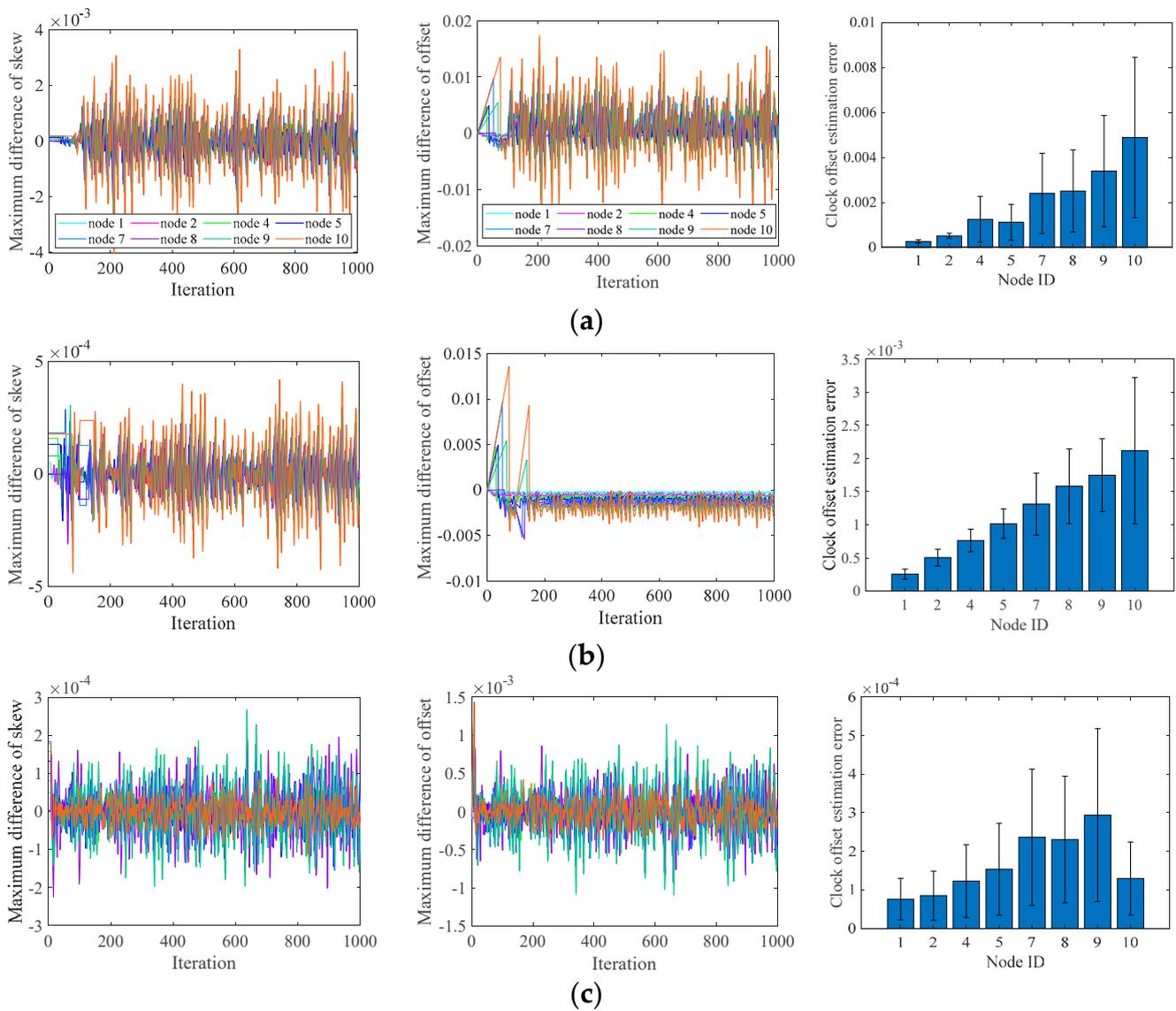
**Figure 6.** Performance of FTSP, FTSP with threshold detection, and RSTS under manipulation attacks. The representation of the lines is the same in (a–c). (a) FTSP; (b) FTSP with threshold detection; and (c) RSTS.
