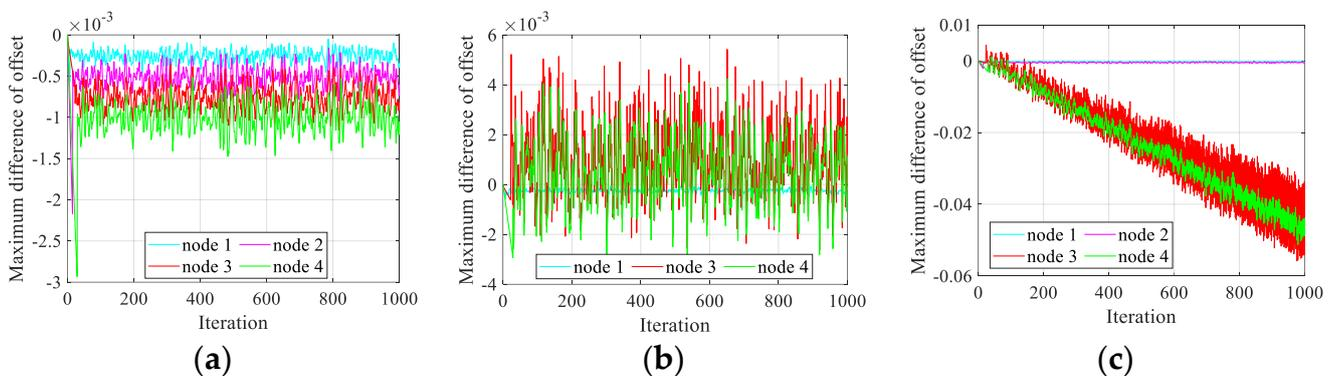
**Figure 2.** Performance of FTSP under various attacks. (a) No attacks; (b) manipulation attacks; and (c) Sybil attacks.
