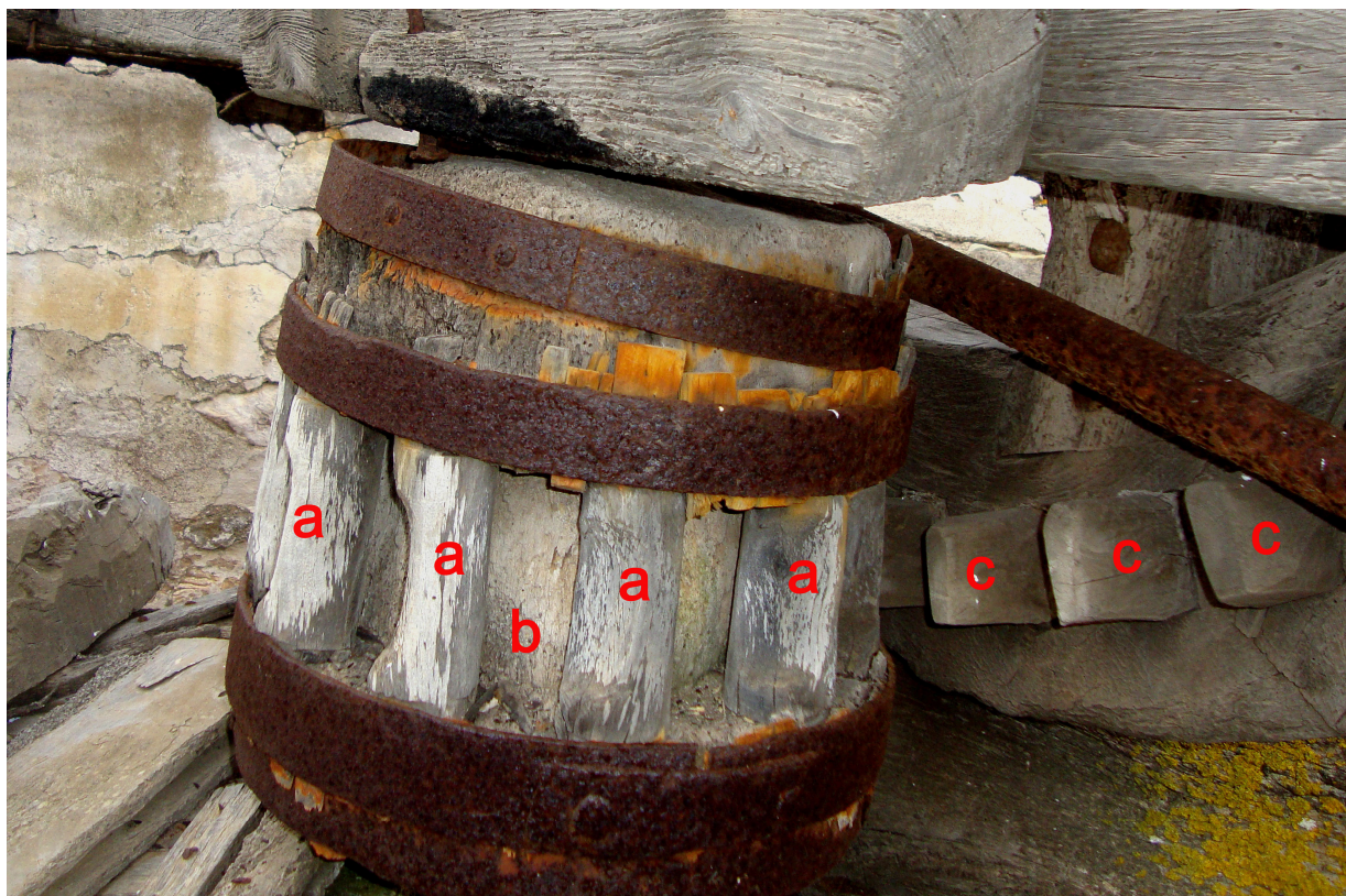
Figure 8. Wallower gear (a. “pentaravda”, b. “anemi”, c. teeth of the brake wheel).
