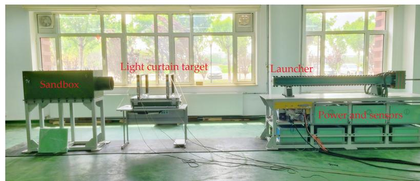
**Figure 17.** The experimental device of the electromagnetic launcher.
