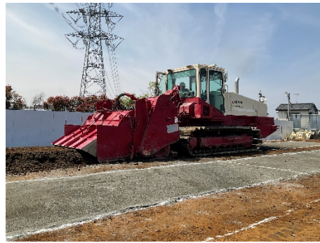
Figure 6. Shallow mixing machine [17] (courtesy of the SHIMIZU CORPORATION).
