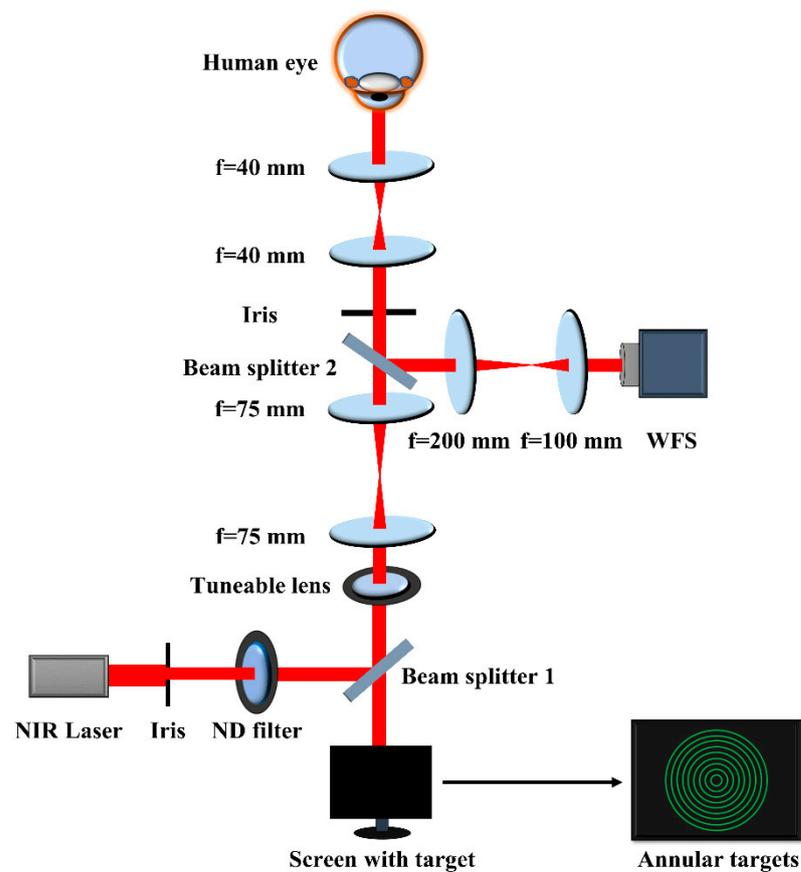
**Figure 1.** Schematic of a monocular vision system which was used to measure foveal, parafoveal and perifoveal accommodation responses to a sequence of random defocus steps. Three 4-f telescopes were used to place the iris, HS-WFS and tunable lens in conjugated pupil planes. Beam splitter 1 is a hot mirror, whereas beam splitter 2 is a 50/50 coated plate. Only a single green ring in the annular accommodation target was shown at any given time.
