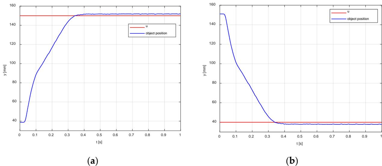
**Figure 8.** Positioning of the object using the cylinder (70%) and the hydraulic motor (30%): (a) upward movement, (b) downward movement.
