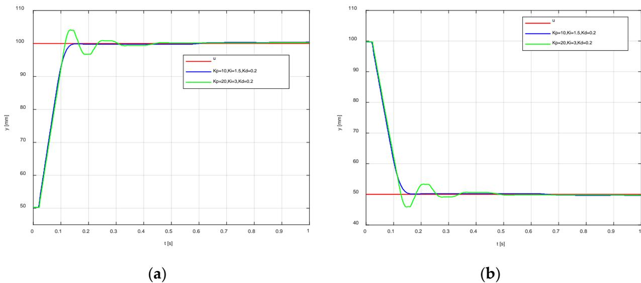
**Figure 6.** Positioning of the hydraulic motor for different set values: (a) upward movement and (b) downward movement.
