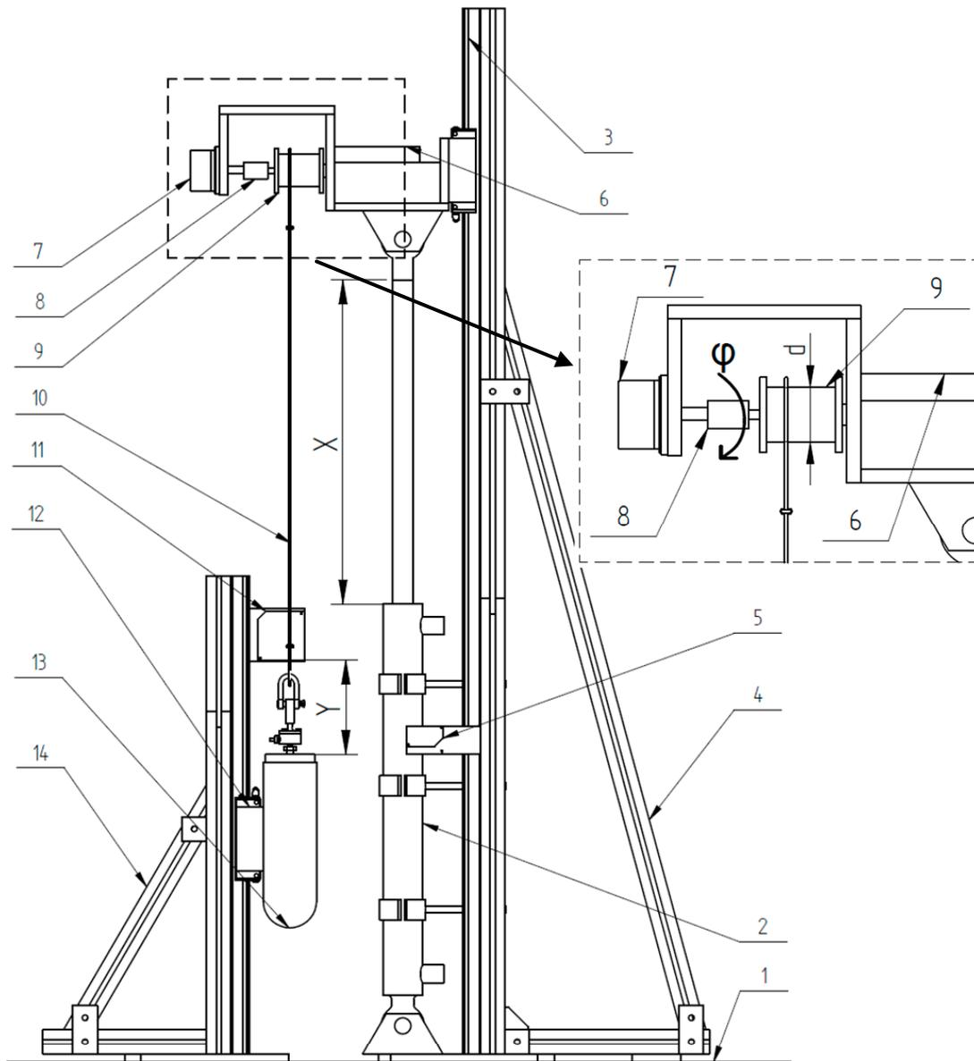
Figure 2. Simplified drawing of the linear rotary electro-hydraulic drive.
