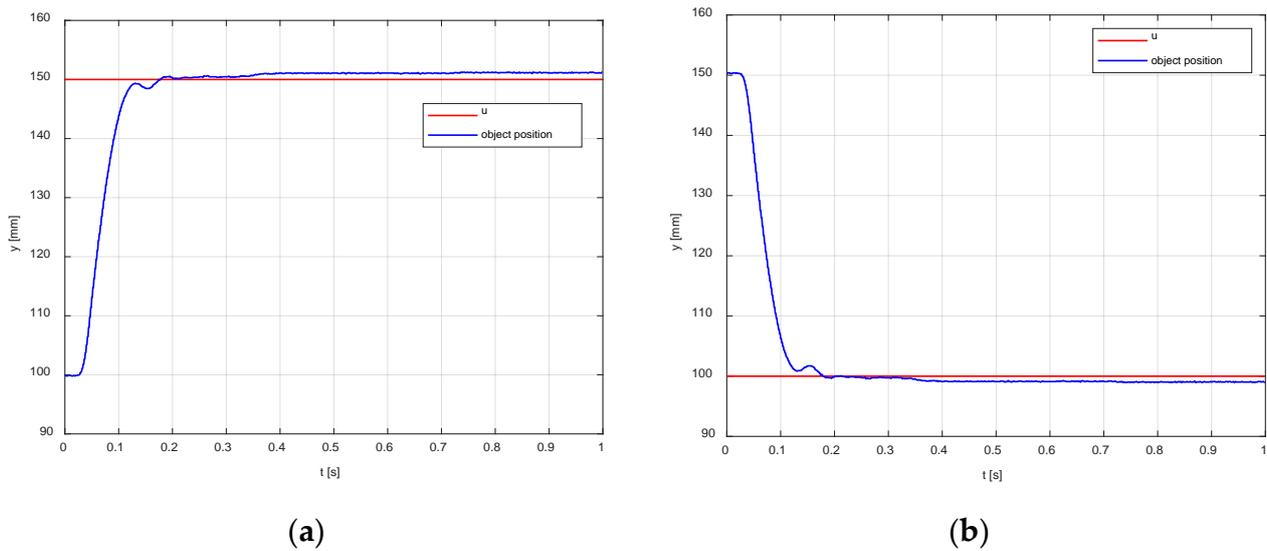
**Figure 7.** Positioning of the object using the cylinder (30%) and the hydraulic motor (70%): (a) upward movement, (b) downward movement.
