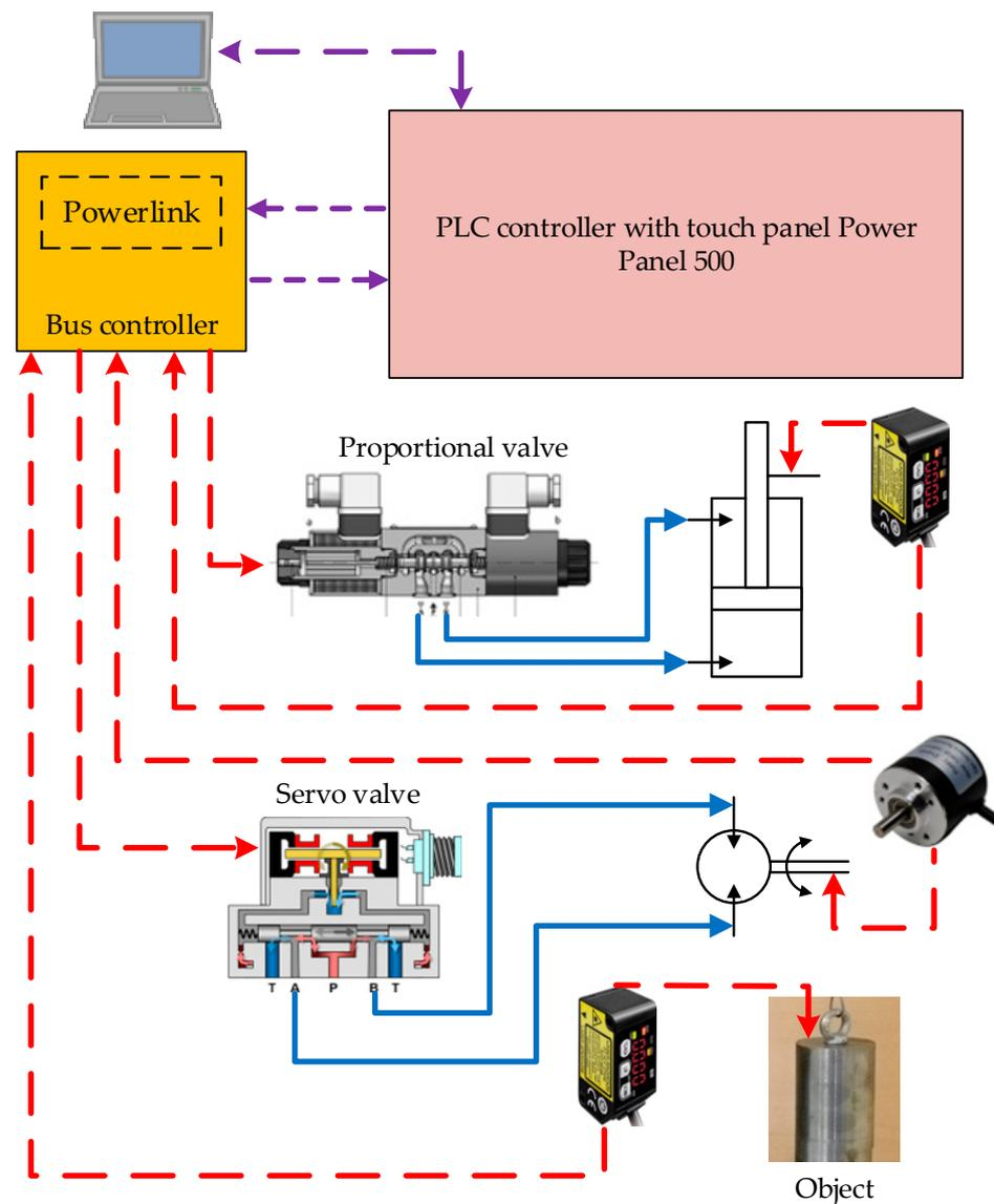
Figure 3. Diagram of the control system.
