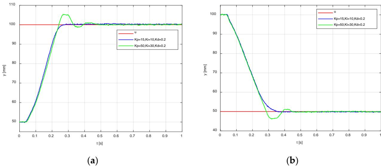
**Figure 5.** Positioning of the cylinder for different parameters of the PID regulator: (a) upward movement, (b) downward movement.
