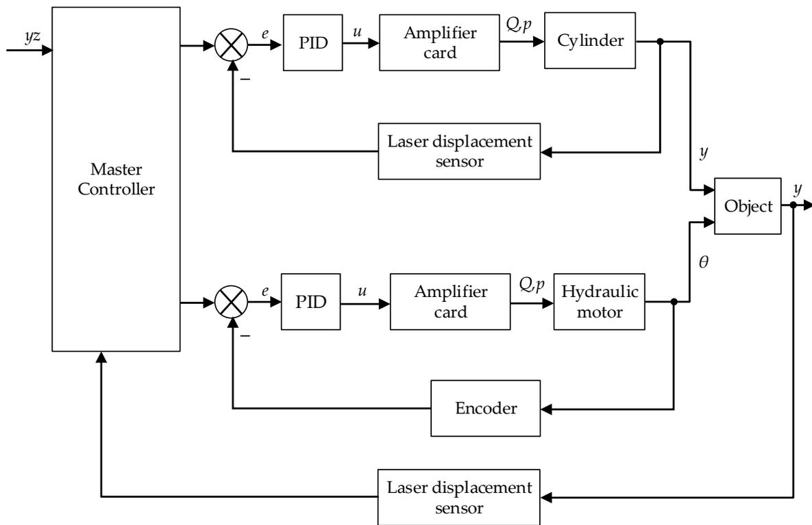
**Figure 1.** Block diagram of the control system for object positioning.
