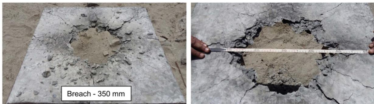
**Figure 8.** Response of the concrete slab to the contact explosion effect [32].
