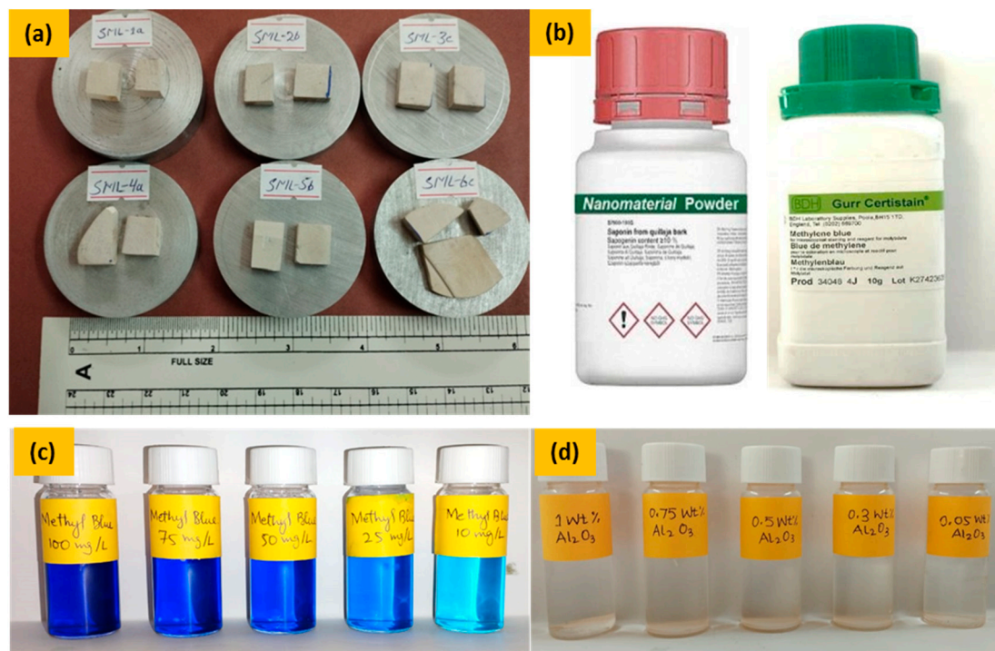
Figure 2. Illustrations of the (a) subsurface carbonate core thin section of Sui main limestone (SML) formation, (b) stack of ( \text{Al}_2\text{O}_3 ) nanoparticle powder and methylene blue dye, (c) MB dye solution under varying concentrations (10, 25, 50, 75, and 100 mg/L, (d) alumina-based nanofluid concentrations (0.05, 0.3, 0.50, 0.75, and 1.0 wt. %).
