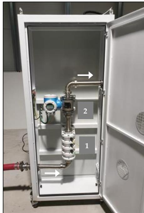
**Figure 2.** PEF equipment picture, including the DN50 treatment chamber (1), flowmeter (2) and the flow of must.
