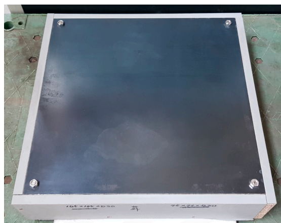
Figure 9. CLP mockup specimen containing concrete voids.
