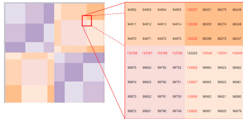
Figure 6. Node map construction for data extraction and reconstruction ( 161 \times 161 pixels).
