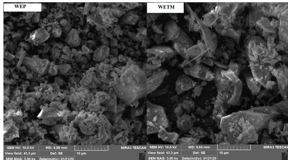
**Figure 4.** FESEM micrographs of the waste vitreous enamel (batch 3).
