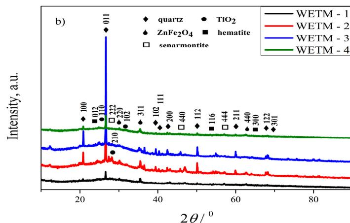
**Figure 2.** XRPD diagrams of the waste vitreous enamels: (a) WEP and (b) WETM.
