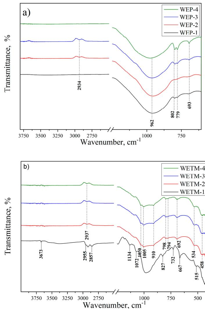
Figure 3. FTIR spectra of the waste vitreous enamels: (a) WEP and (b) WETM.
