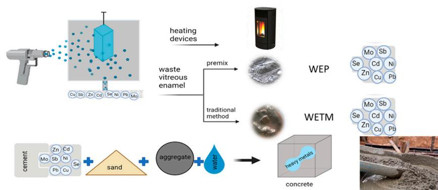
**Figure 1.** The representative samples of raw waste vitreous enamel samples and their use for cement partial replacement in the concrete and mortar production.
