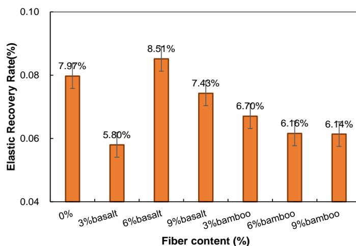
Figure 22. Elastic recovery rate of asphalt mastics.
