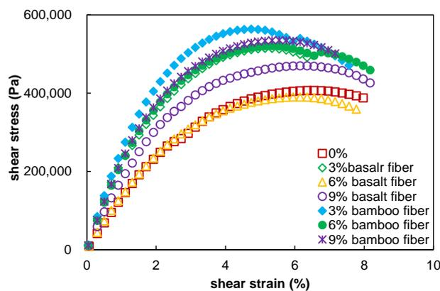
Figure 12. Curves illustrating the relationship between strain and stress in fiber-modified asphalt mastics.
