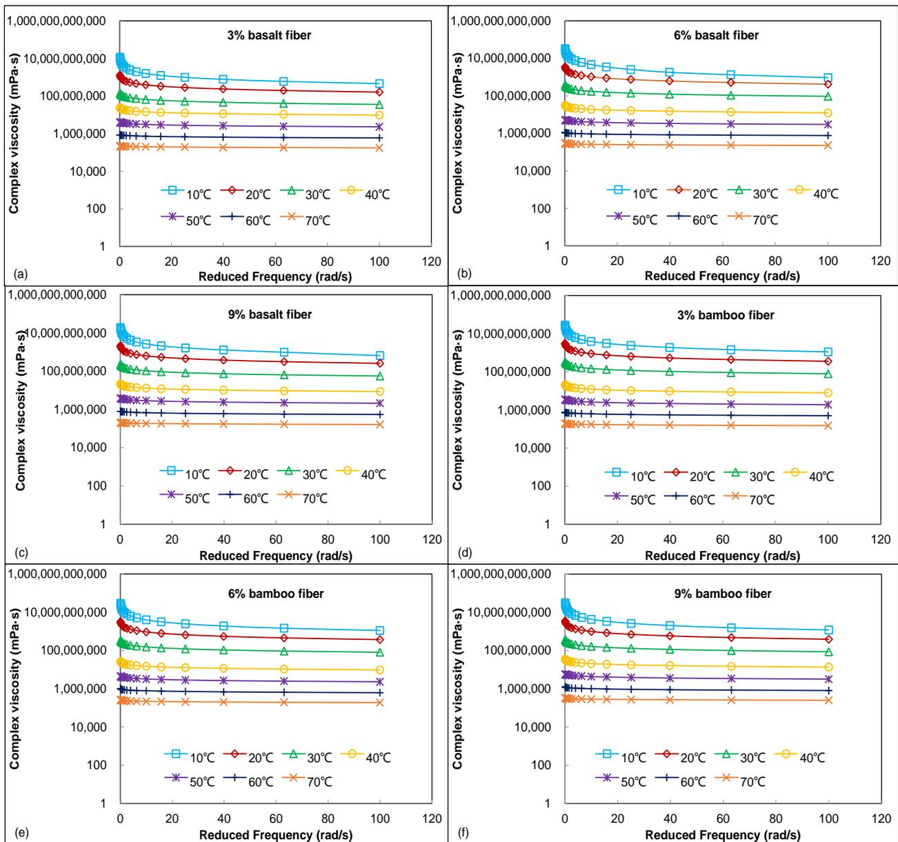
**Figure 10.** Viscosity results of modified asphalt mastic: (a) 3% basalt fiber; (b) 6% basalt fiber; (c) 9% basalt fiber; (d) 3% bamboo fiber; (e) 6% bamboo fiber; (f) 9% bamboo fiber.
