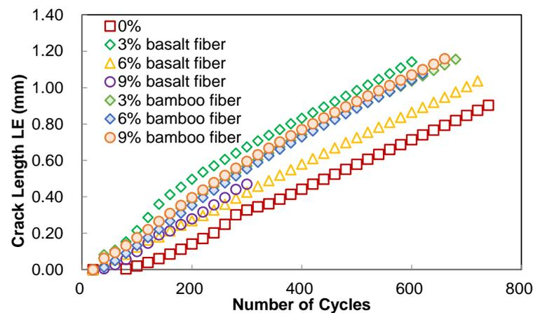
Figure 18. Crack length summary of fiber modified asphalt mastic.
