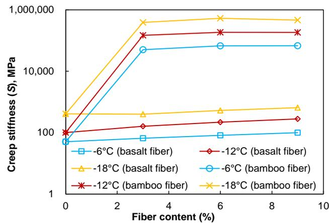
Figure 23. Creep stiffness of fiber-modified asphalt mastics.
