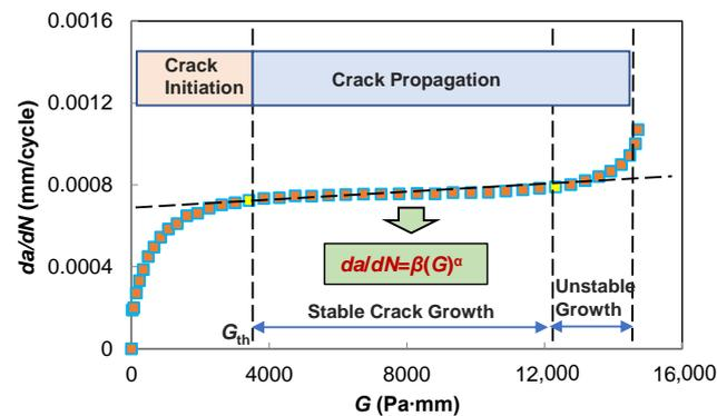
Figure 16. This pertains to the correlation between the rate of cracking ( $da/dN$ ) and the energy release rate ( $G$ ).
