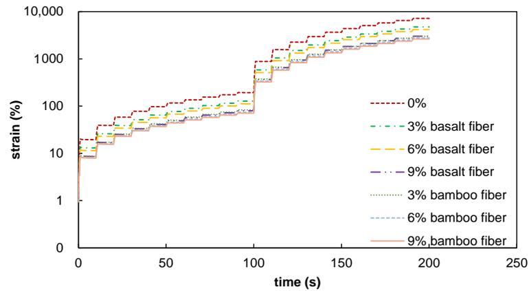
Figure 19. Time–strain curves of different types of fiber-modified asphalt mastics.
