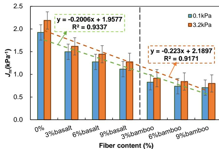
Figure 20. Effect of fiber modification on asphalt mastic  $J_{nr}$  values.
