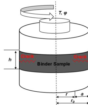
Figure 15. A diagrammatic representation for the calculation of asphalt binder crack length [32].
