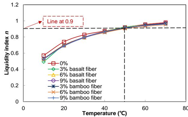
Figure 11. Evaluation of flow characteristics index in fiber-modified asphalt mastics.
