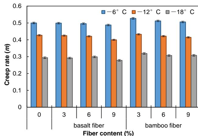
Figure 24. Effects of fiber modification on creep rate of asphalt mastics.
