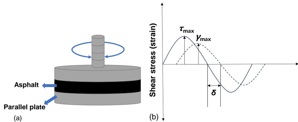
Figure 2. Schematic diagram of the tests: (a) operational principle of DSR; (b) wave pattern of stress and strain.
