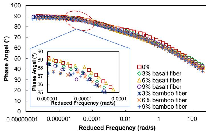
**Figure 7.** Master curves of phase angle for various types of fiber-modified asphalt mastic.
