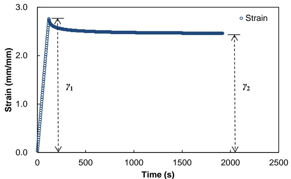
Figure 5. Time–strain results model based on ER test.
