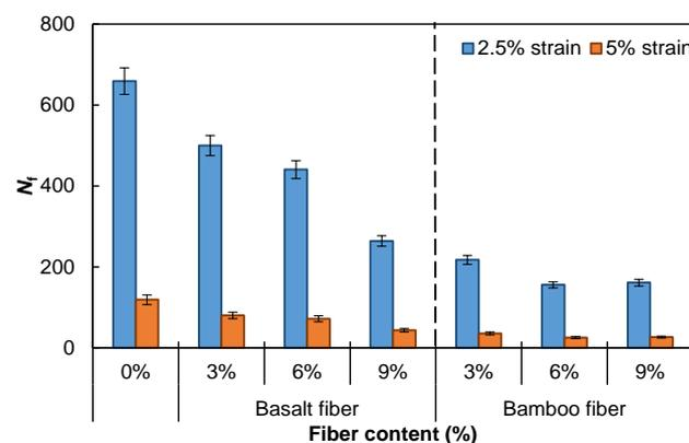
Figure 14. Fatigue life evaluation of asphalt mastics modified with fibers.
