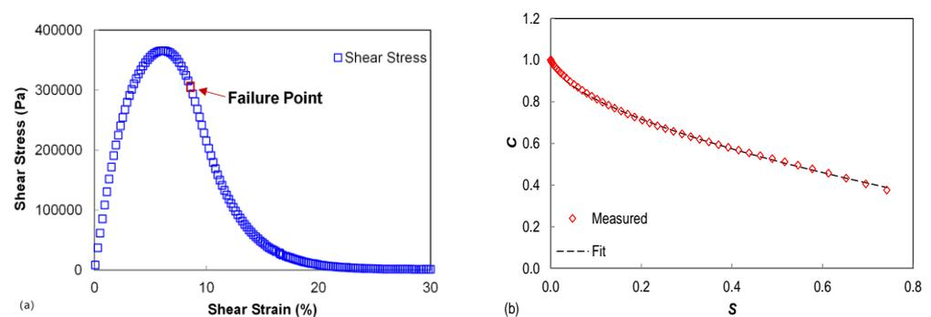
**Figure 4.** Modification of the fatigue model of the base asphalt binder at 20 °C by incorporating LAS data: (a) stress–strain curve; (b) damage characteristic curve.
