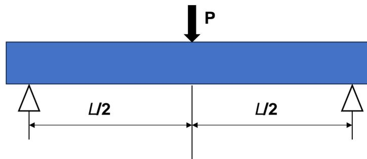
Figure 3. Schematic diagram of BBR test.
