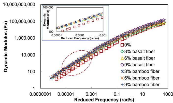
**Figure 6.** Master curves displaying the dynamic modulus for various types of fiber-modified asphalt mastic.
