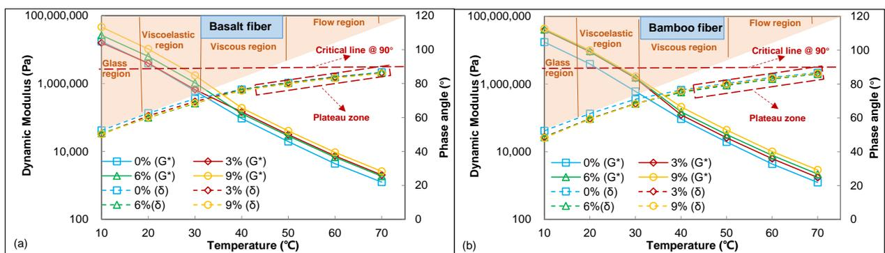
Figure 9. Temperature's effect on fiber-modified asphalt mastics' modulus and phase angle: (a) basalt fiber; (b) bamboo fiber.
