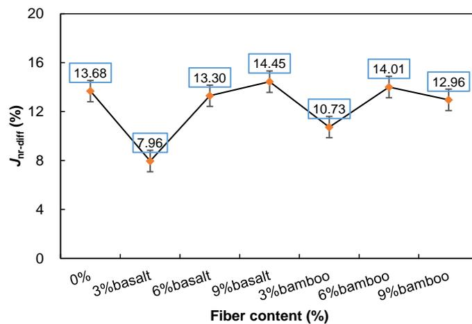
Figure 21. Effect of fiber modification on asphalt mastic  $J_{nr-diff}$ .
