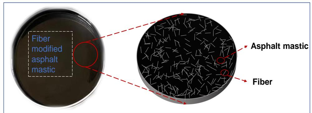
Figure 8. Illustration of asphalt mastic sample.
