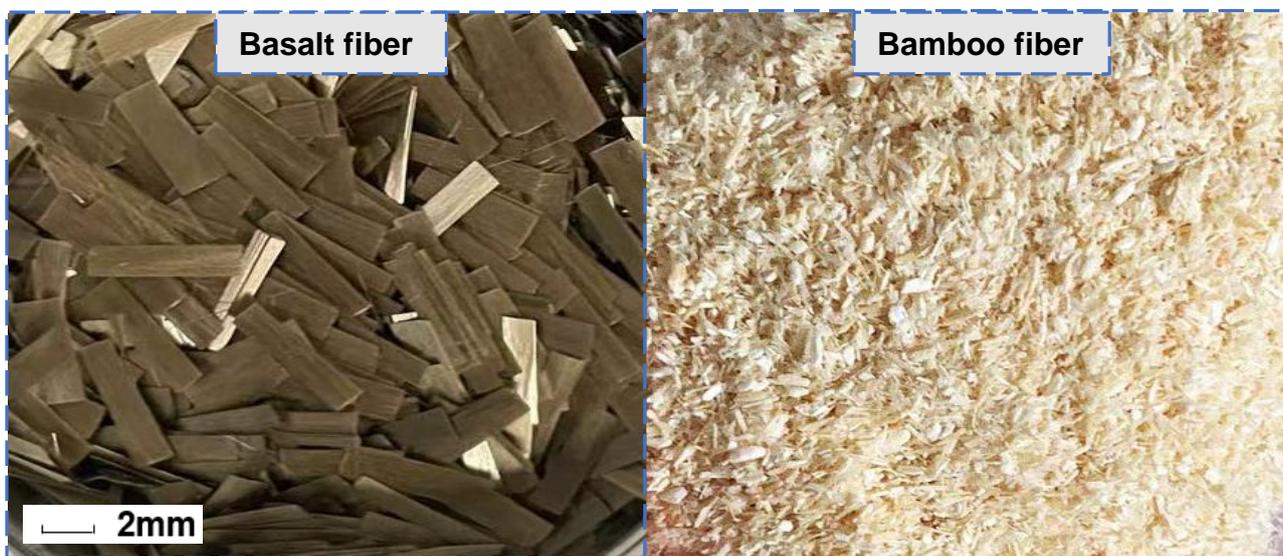
**Figure 1.** Basalt and bamboo fiber morphology.
