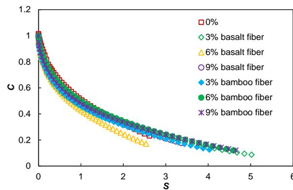
Figure 13. Effects of fiber incorporation on the  $C$  vs.  $S$  curves of asphalt mastics.
