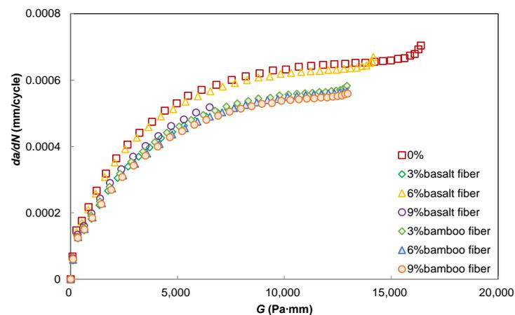
Figure 17. Diagram showing two-phase crack growth in an LAS test.
