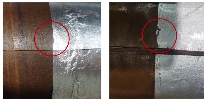
Figure 2. Bushing foil layer breakage defects.
