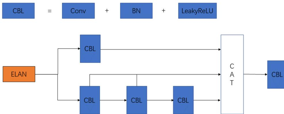
Figure 4. YOLOv7tiny ELAN.
