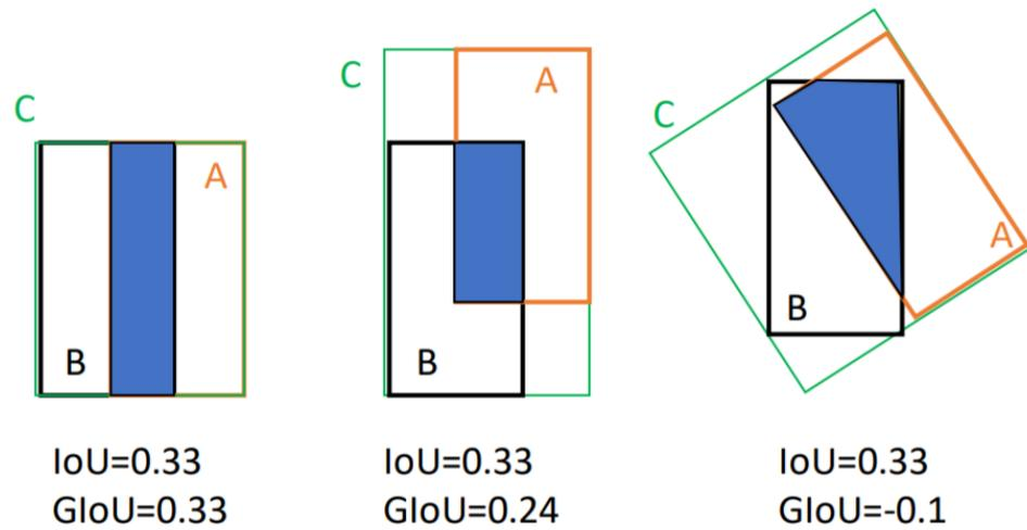
Figure 6. Different ways of overlapping detection frames.
