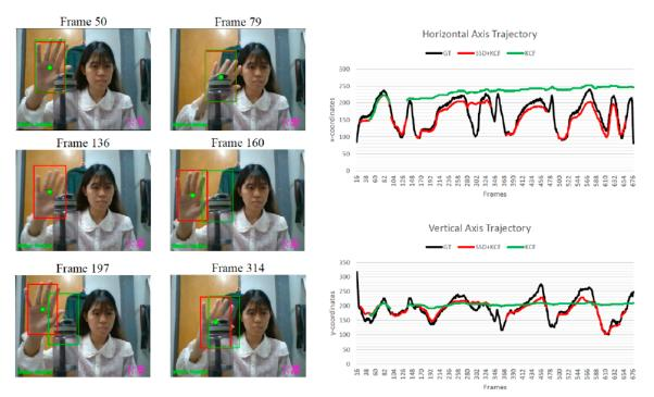
**Figure 4.** Tracking results of proposed algorithm (red) and KCF tracker (green) on occluded hand behind other object.
