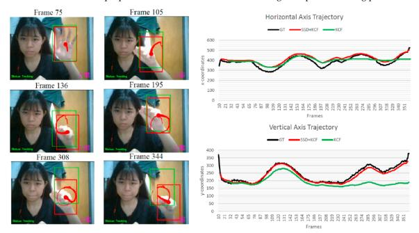
**Figure 6.** Tracking results of proposed algorithm (red) and KCF tracker (green) on deformable hand shape.
