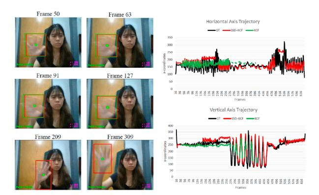
**Figure 3.** Tracking results of proposed algorithm (red) and KCF tracker (green) for tracking fast hand movement.
