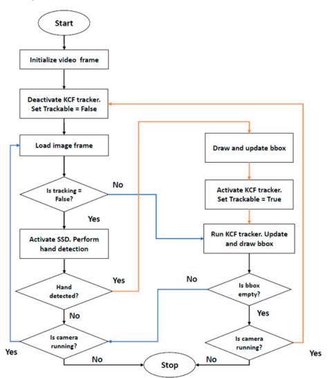
Figure 1. Flowchart of the integration of SSD and KCF Tracker.
