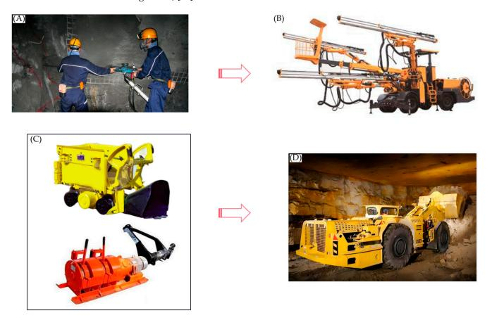
Figure 3. (A) Pneumatic rock drill; (B) Rock drill cart; (C) Electric rake and rock loader; (D) LHD.
