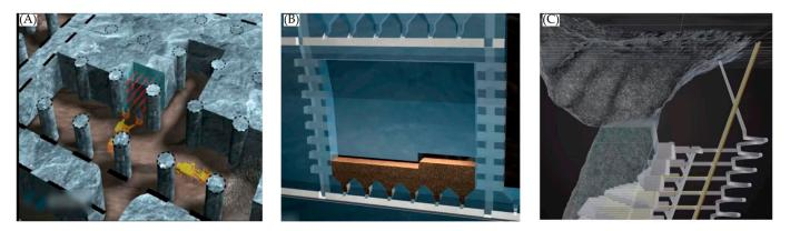
**Figure 2.** (**A**) Schematic diagram of room-and-pillar method; (**B**) Schematic diagram of shrinkage stoping mining method; (**C**) Schematic diagram of sublevel caving mining method.
