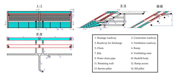
Figure 8. Shishudi Gold Mine: Schematic diagram of the upward horizontal cut and backfill stoping method.
