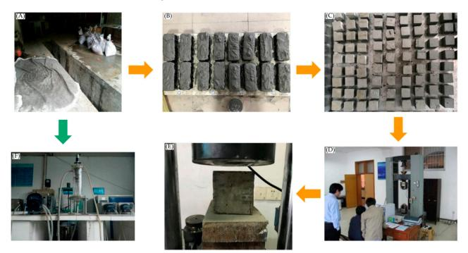
**Figure 7.** Shishudi Gold Mine backfill experiments: (**A**) Tailings sampling; (**B**) Test blocks making; (**C**) Test blocks finishing; (**D**) Compression testing equipment; (**E**) Compression test; (**F**) Simulation experiment: deep-cone thickener.
