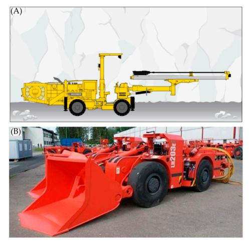
Figure 10. Shishudi Gold Mine: (A) Hydraulic rock drilling trolley, type: Boomer K41; (B) LHD.
