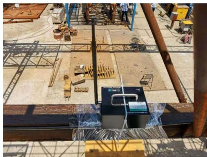
Figure 14. JM3874 accelerometer.
