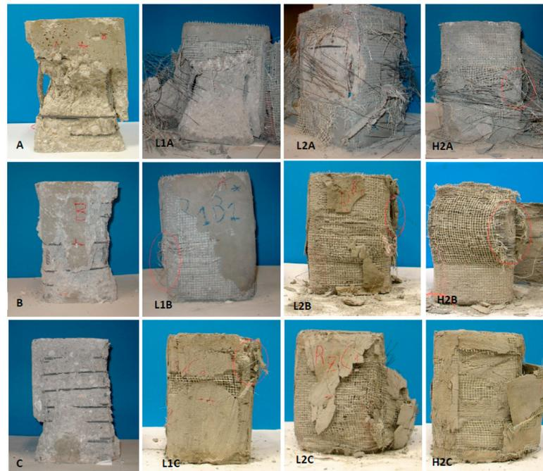
**Figure 5.** Control (X = A, B, C) and SRG-jacketed columns (DiX) at failure.
