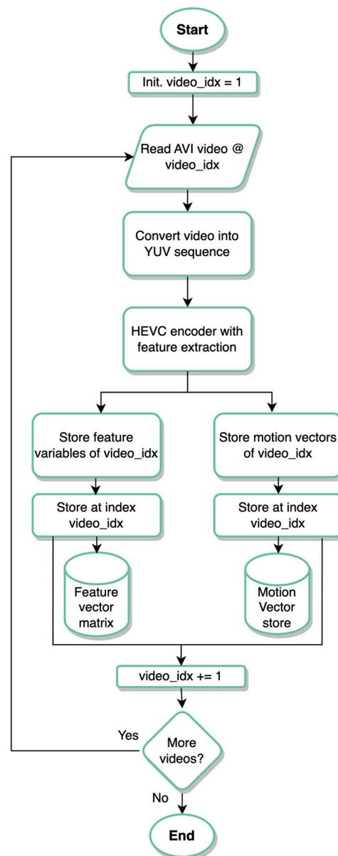
**Figure 2.** Flowchart of overall proposed feature extraction.
