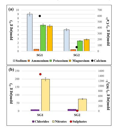
**Figure 2.** Ion concentration of samples SG\_1 and SG\_2 taken from Panel E. (a) Ppm ( $\mu$ g g<sup>-1</sup>) concentrations of sodium, ammonium, potassium, magnesium and calcium cations; (b) ppm concentrations ( $\mu$ g g<sup>-1</sup>) of chloride, nitrate and sulphate ions.
