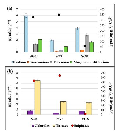
**Figure 4.** Ion concentration of samples SG\_6, SG\_7 and SG\_8 taken from Panel A. (a) Ppm ( $\mu$ g g<sup>-1</sup>) concentrations of sodium, ammonium, potassium, magnesium and calcium cations; (b) ppm concentrations ( $\mu$ g g<sup>-1</sup>) of chloride, nitrate and sulphate anions.
