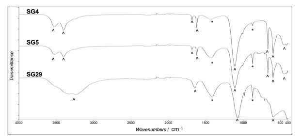
**Figure 7.** ATR-FTIR spectra of samples SG\_4, SG\_5 and SG\_229 taken from Panel C. Marker bands of carbonates (\*) and sulphates (^) are highlighted.
