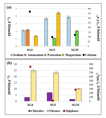
**Figure 6.** Ion concentrations of samples SG\_4, SG\_5 and SG\_29 taken from Panel C. (a) Ppm ( $\mu$ g g<sup>-1</sup>) concentrations of sodium, ammonium, potassium, magnesium and calcium cations; (b) ppm concentrations ( $\mu$ g g<sup>-1</sup>) of chloride, nitrate and sulphate anions.
