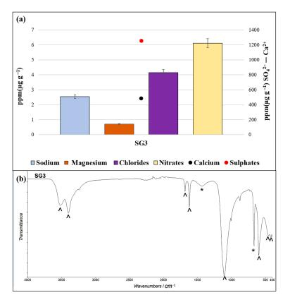
**Figure 8.** Sample SG3 taken from Panel D. (a) Ion concentrations of sodium, magnesium, chlorides, nitrates, calcium, sulphate in ppm ( $\mu$ g g<sup>-1</sup>); (b) ATR-FTIR spectrum: marker bands of carbonates (\*) and sulphates (^) are highlighted.
