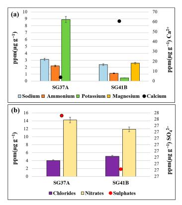
Finally, samples taken at the top of the vault do not show high values of sulphate and calcium ions (moderate concentrations were only obtained in sample SG\_37A) (Figure 9).
