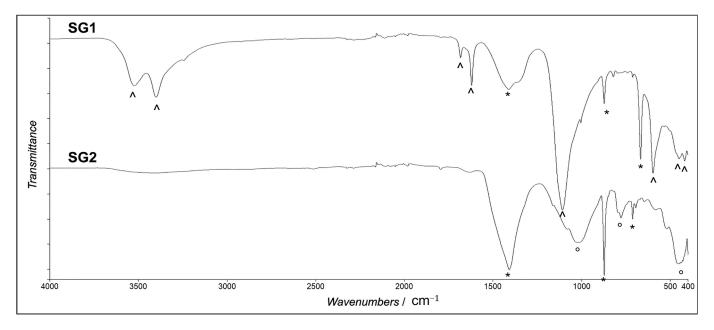
**Figure 3.** ATR-FTIR spectra of samples SG\_1 and SG\_2 taken from Panel E. Marker bands of carbonates (\*), silicates (°) and sulphates (^) are highlighted.
