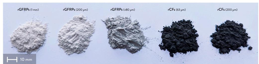
**Figure 1.** Mechanically recycled glass fibers and mechanically and thermally carbon fibers used in this work (from left to right): rGFRPs (1 mm, 200  $\mu\text{m}$ , <80  $\mu\text{m}$ ) and rCFs (63  $\mu\text{m}$ , 200  $\mu\text{m}$ ).
