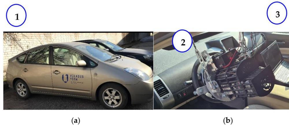
**Figure 8.** (a) The prototype of the first-level autonomous ground vehicle. (b) The automated steering device with the control computer.
