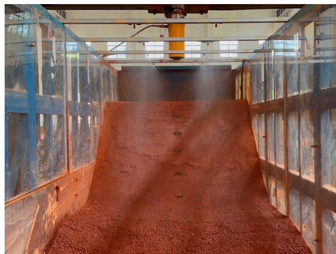
Figure 5. Rainfall simulation system.
