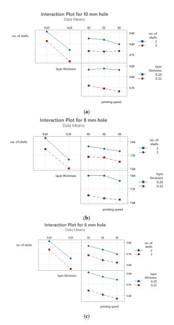
**Figure 5.** Interaction plots for the holes dimensional accuracy (a) 10 mm holes; (b) 8 mm holes; (c) 6 mm holes.
