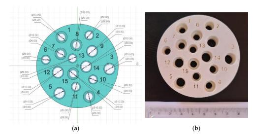
**Figure 2.** 3D CAD model of test part 1 (a); Example of a test part with counterbore vertical axis holes for the experiment 1 (specimen 16) (b).
