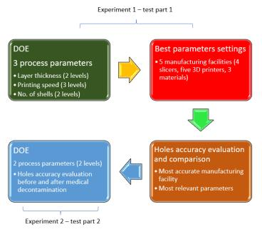
Figure 1. Schematic representation of the research methodology.
