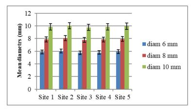
**Figure 6.** Mean diameter values for tests parts built using different 3D printers, materials and slicing software.
