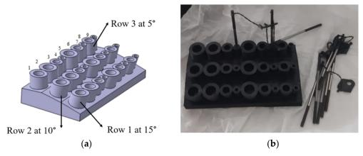
**Figure 3.** Test part 2 with holes of 2.3 mm, 4.5 mm, and 6.5 mm in diameter (holes axes angles of  $5^{\circ}$ ,  $10^{\circ}$  and  $15^{\circ}$ ): (a) virtual model, (b) pass-no pass test on the physical model.
