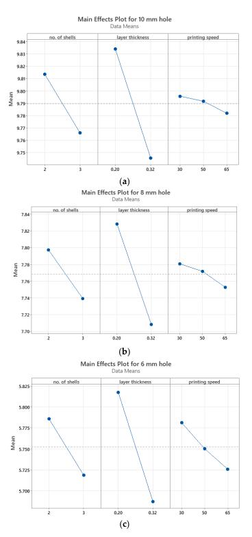
**Figure 4.** Main effect plots for the holes dimensional accuracy: **(a)** 10 mm holes; **(b)** 6 mm holes; **(c)** 8 mm holes.
