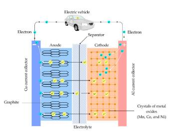
**Figure 11.** Lithium ions flow from the anode to the cathode and push electrons to flow within outside circuit. The electric vehicle charges in the reverse process. Adapted from [89,90].
