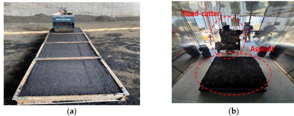
Figure 6. (a) Preparation of asphalt concrete specimen and (b) chamber experimental setup.
