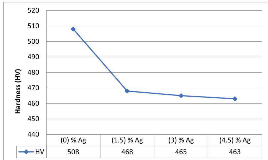
**Figure 5.** Micro-hardness (Hv) of Ti-Ni-Ag alloys.
