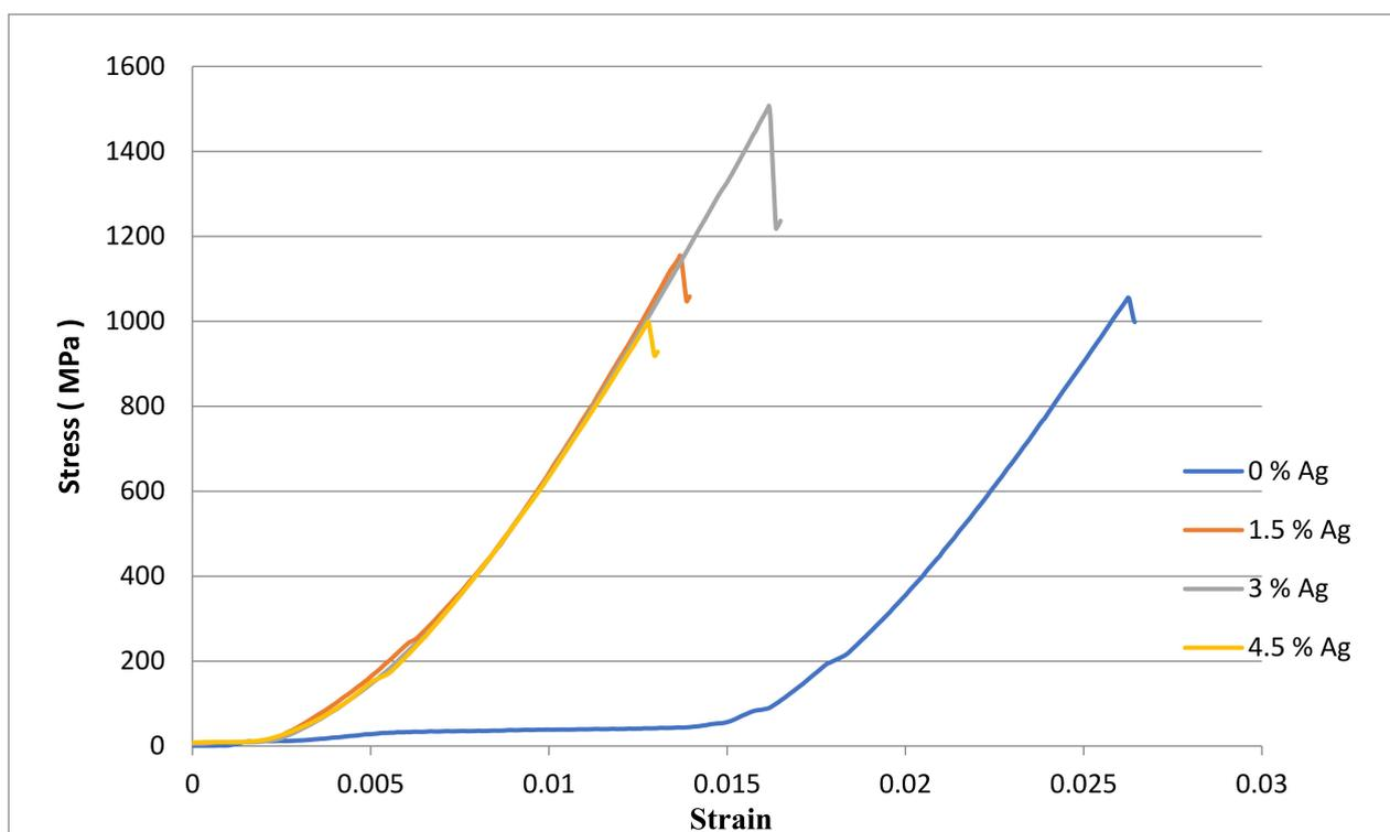
**Figure 4.** Compressive stress–strain curves of the Ni-Ti-Ag samples.
