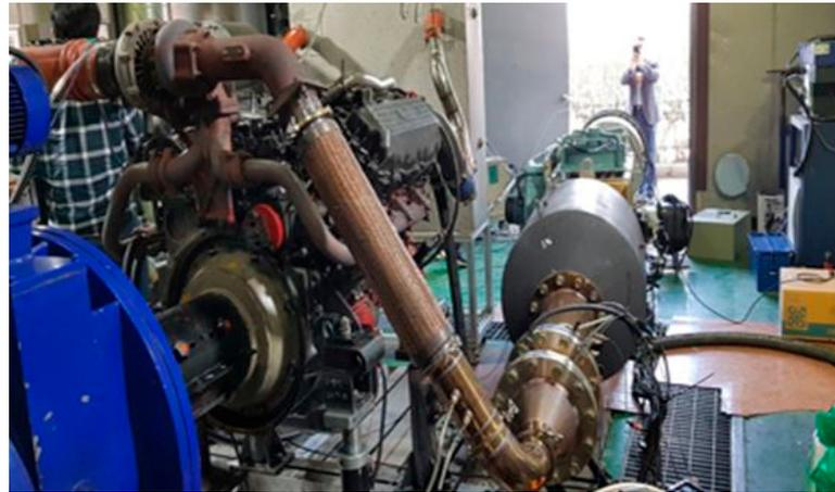
**Figure 14.** Back pressure test rig: circle-type system.
