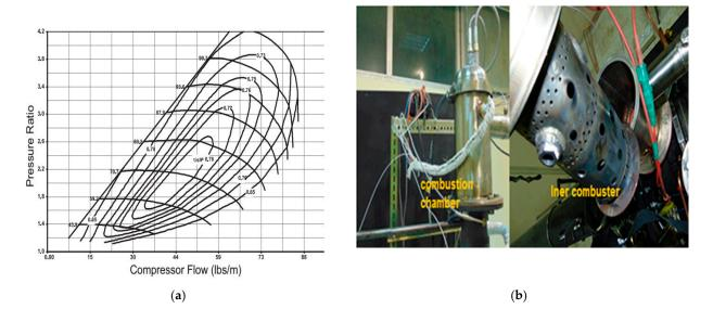
Figure 3. Fabricated GTE (a) compressor map and (b) adapted combustion chamber.
