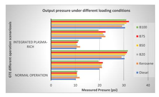
Figure 9. Compressor output pressure comparison plot.
