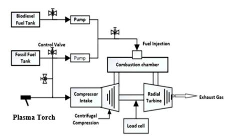
Figure 2. Schematic diagram of the fabricated micro gas turbine engine.
