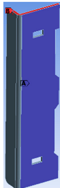
Figure 5. Support subjected to random vibration fatigue.
