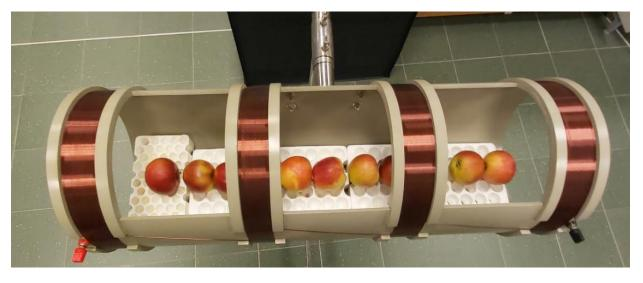
Figure 1. Coil designed for fruit storage in room conditions.
